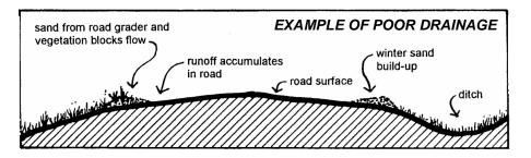
**Ditch shape**: the shape of the ditch should be a rounded-V. The side slopes of the ditch should not be steeper than a 1.5:1 slope.
