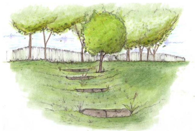
Figure 2. Check dams within a swale slow the flow, allowing sediments to settle out and some infiltration to occur.
